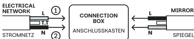
**TO ENSURE COMPLIANCE WITH IP44 SAFETY, IT IS ESSENTIAL TO USE THE CONNECTION BOX TO PERFORM THE FOLLOWING STEPS:**
